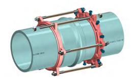
2 Complete the pipe joint assembly per the pipe manufacturer instructions, Position restraint ring on spigot end of pipe by inserting one of the restraint rods into the restrainer ears of restraint ring and harness ring so that the restraint rod ends extend past each nut approximately 1/2". Complete inserting the remaining restraint rods through the restrainer ears. Only hand-tighten all the hex nuts at this point.
