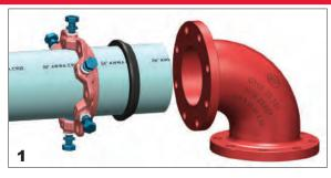
**1** Check the EZ Grip Restrained Flange Adapter for any missing components and any damage. Also be certain the O-ring gasket on the flange face is properly seated in its raceway.
