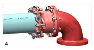
**4** Tighten the T-Bolts to normal range of bolt torque per table below. T-bolts should be tightened alternately on opposite sides using a 'Star Pattern'. It is important that the gland be brought up toward the bell socket evenly, maintaining approximately the same distance between the gland and the face of the bell socket at all points around the socket.
