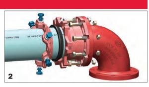
**2** Apply approved pipe lubricant to both the M.J. gasket and the plain end of pipe that meets the AWWA C151 Standard. Slide the MJ gasket over the pipe with the beveled edge towards the MJ bell of Adapter.
