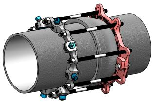
**3** Position the EZ Grip wedge gland on spigot end of pipe by inserting the restraint rods into the restrainer ears of the split ring follower so that the threaded rod ends extend past the ear. Thread a nut on the rod so that ½" of threads are seen on both ends of the rods. Only had tighten all hex nuts at this time
