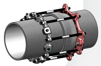
**4** Hand adjust the nuts on the rod to ensure at least ½" of threads are exposed but that the rods are evenly against both the EZ Grip wedge gland and the split ring follower.
