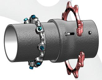
**2** While pipe ends are still apart slide the EZ Grip wedge gland over the plain end of the pipe with the lip facing the spigot end of the pipe. Assemble the split ring follower on the back side of the pipe bell with flat side of bolt ears facing away from the bell. Tighten the split ring follower bolts on each side until bolt and nut are securely fastened. Complete the pipe joint assembly per the pipe manufactures recommendations.
