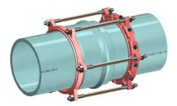
4 Hand-tighten all nuts so that the rods stick out approximately 1/2" past the nuts. Make sure that the solid harness ring is evenly bearing against the pipe bell.
