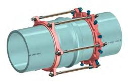
3 Tighten down the break-off torque nuts until all the wedges are in firm contact with the pipe surface. Once this step is completed, continue tightening in an alternate manner ('star' pattern) until all the break-off torque nuts have sheared off. A 5/8" hex-head will remain, if disassembly is necessary. See Torque ranges below\*
