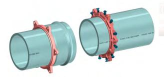
1 Clean and prepare the pipe for installation using normal procedures per pipe manufacturer. Slide the EZ GRIP® PTP restraint gland, with lip facing spigot end, onto the first pipe. Next slide the solid harness ring along the length of second pipe and fit closely behind the pipe bell.
