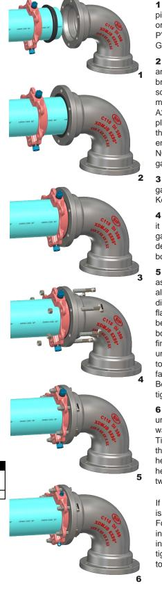
**1** Establish the type and diameter of the PVC pipe. If the PVC pipe is AWWA C900, C905, or C909 then a Standard gasket is used. If the PVC pipe is IPS (Steel OD) then a Transition Gasket is required for proper sealing.
