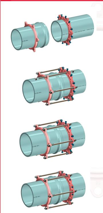
1 Clean and prepare the pipe for installation using normal procedures per pipe manufacturer. Slide the EZ GRIP® PTP restraint gland, with lip facing spigot end, onto the first pipe. Next slide the solid harness ring along the length of second pipe and fit closely behind the pipe bell.
