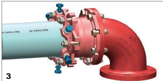
**3** Center the pipe evenly into the I.D. of the Adapter and slide the MJ Gasket into the MJ bell recess of the Adapter. Slide the EZ Grip towards the Adapter with the Gland lip against the gasket. Insert T-bolts and hand-tighten nuts.
