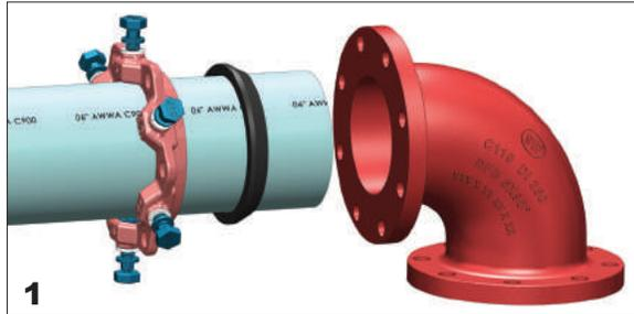
**1** Check the EZ Grip Restrained Flange Adapter for any missing components and any damage. Also be certain the O-ring gasket on the flange face is properly seated in its raceway.
