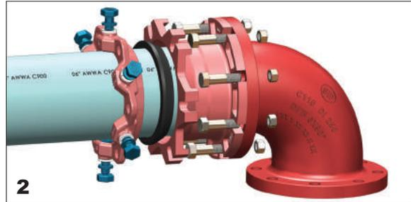
**2** Apply approved pipe lubricant to both the M.J. gasket and the plain end of pipe that meets the AWWA C151 Standard. Slide the MJ gasket over the pipe with the beveled edge towards the MJ bell of Adapter.
