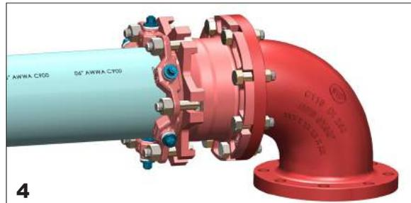
**4** Tighten the T-Bolts to normal range of bolt torque per table below. T-bolts should be tightened alternately on opposite sides using a 'Star Pattern'. It is important that the gland be brought up toward the bell socket evenly, maintaining approximately the same distance between the gland and the face of the bell socket at all points around the socket.
