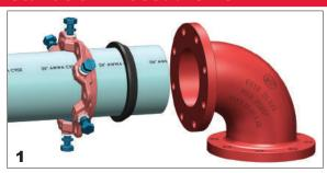
**1** Check the EZ Grip Restrained Flange Adapter for any missing components and any damage. Also be certain the O-ring gasket on the flange face is properly seated in its raceway.
