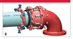
**2** Apply approved pipe lubricant to both the M.J. gasket and the plain end of pipe that meets the AWWA C151 Standard. Slide the MJ gasket over the pipe with the beveled edge towards the MJ bell of Adapter.
