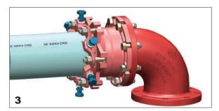
**3** Center the pipe evenly into the I.D. of the Adapter and slide the MJ Gasket into the MJ bell recess of the Adapter. Slide the EZ Grip towards the Adapter with the Gland lip against the gasket. Insert T-bolts and hand-tighten nuts.
