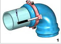
**1** Insert the gasket and PVC pipe into PVC fitting using the manufacturer's instructions. Next, install the two non-serrated gland halves on the bell of the fitting and tighten the clamping bolts to the recommended torque level given in the table below. Then, insert one of the long T-bolts / threaded rods through one of the bolt holes and mark a line approximately 2 inches from the far end of the bolt/rod (towards the fitting)
