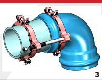
**3** Assemble the remaining T-bolts/rods through the retaining ring and the restraining ring and tighten for a snug fit
