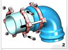
**2** Using the T-bolts/rods as guides, assemble the serrated gland halves on the pipe with the far side of the gland in line with the mark on the pipe. Then, tighten the clamping bolts to the given torque levels (see table below).
