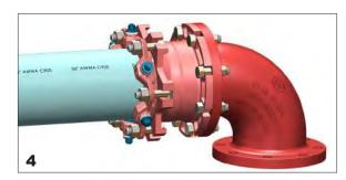
**4** Tighten the T-Bolts to normal range of bolt torque per table below. T-bolts should be tightened alternately on opposite sides using a 'Star Pattern'. It is important that the gland be brought up toward the bell socket evenly, maintaining approximately the same distance between the gland and the face of the bell socket at all points around the socket.
